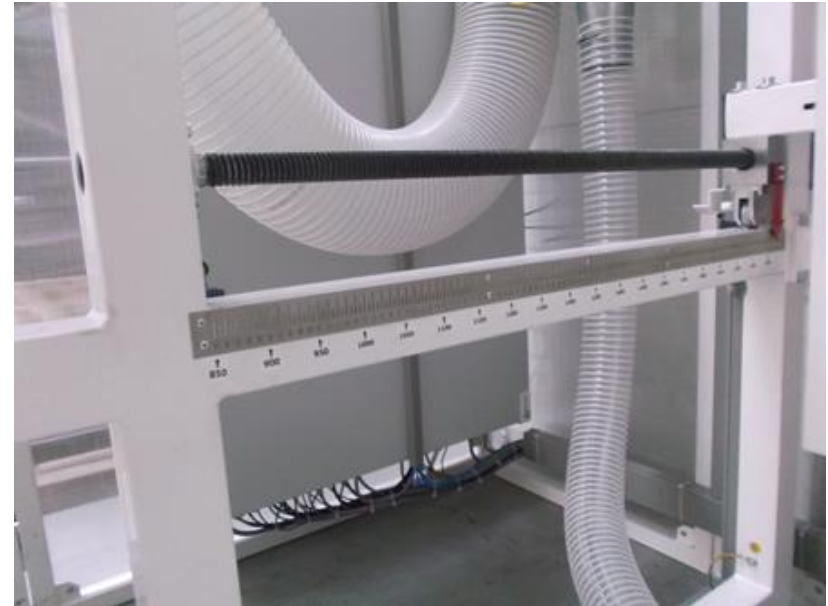
Measuring the distance from the wall and blade saw.
