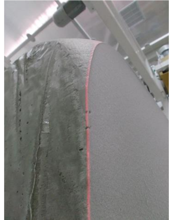
Line laser for marking the position of the cut.
