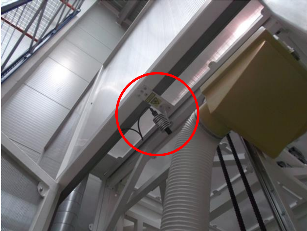
Line laser for marking the position of the cut.
